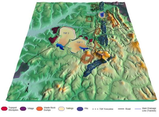
Figure 18.4 – General Arrangement of the Lola Mine Site (2019)
