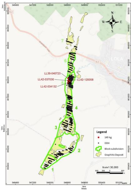
Figure 13.6 – Map of the Lola Deposit showing the Location of Hard Rock Samples
