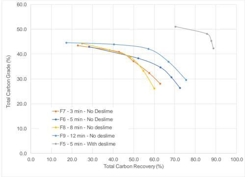
Figure 13.2 - Rougher Flotation Test Results With and Without Desliming
