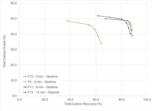
Figure 13.3 – Rougher Flotation Tests with Increasing Scrubbing Time
